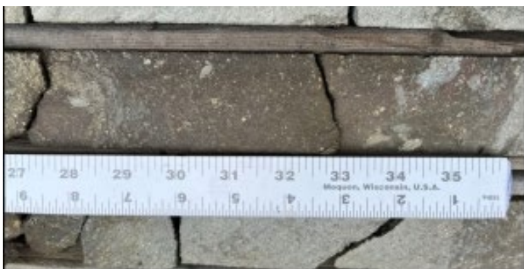
Drillhole 102509: Remobilized, brecciated massive sulphide hosted by Pipe Formation (Thompson Mine Sequence): 0.98% Ni over 32.61 m incl. 3.49% over 2.23 m
