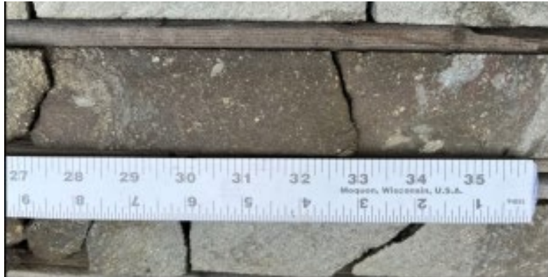
Drillhole 102509: Remobilized, brecciated massive sulphide hosted by Pipe Formation (Thompson Mine Sequence):
