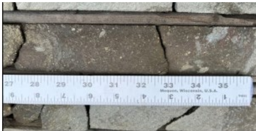
Allochthonous, brecciated massive sulphide hosted by Pipe Formation metapelite containing metapelite clasts, drill hole 102509
